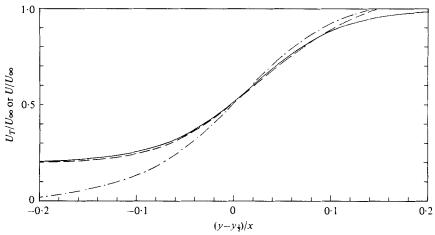
FIGURE 4. Temporal and conditional turbulent mean velocity profile as measured by Wygnanski & Fiedler (1970). ---, mean velocity profile,  $U/U_{\infty}$ ; ---, conditional turbulent mean velocity profile,  $U_T/U_{\infty}$ ; ---, equation (2.3),  $\eta = \sigma(y - y_{\frac{1}{2}})/x - 0.22$ ,  $y_{\frac{1}{2}} = \text{location where } U/U_{\infty}$  is 0.5.
