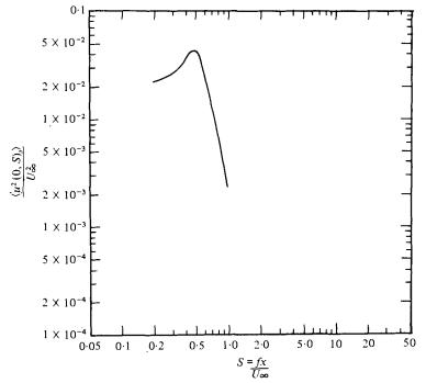
FIGURE 18. Power spectrum of longitudinal turbulent velocity fluctuations associated with the large structures of two-dimensional mixing layers on the plane y = 0.
