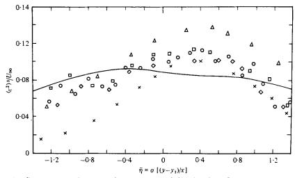
FIGURE 14. Comparison of measured and computed distribution of root-mean-square transverse turbulent velocity fluctuations. Patel (1973):  $\diamondsuit$ , x = 28 cm;  $\Box$ , x = 65.3 cm;  $\bigcirc$ , x = 102.5 cm.  $\triangle$ , Wygnanski & Fiedler (1970);  $\times$ , Liepmann & Laufer (1947); -----, present calculation.
