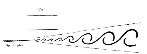
FIGURE 1. A stretch of large structures in a two-dimensional mixing layer.
