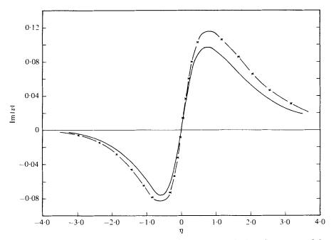
FIGURE 8. Effect of turbulent Reynolds number on the imaginary part of the eigenfunction,  $\bar{\alpha} = 0.5$ ,  $\bar{\omega} = 0.425$ . ....,  $R_T = 500$ ; ×--×,  $R_T = \infty$ .
