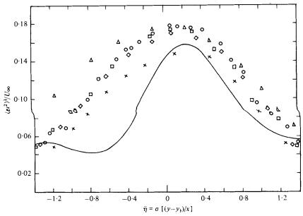
FIGURE 15. Comparison of measured and computed distribution of root-mean-square longitudinal turbulent velocity fluctuations. Patel (1973):  $\diamondsuit$ , x = 28 cm;  $\Box$ ,  $x = 65\cdot3$ ;  $\bigcirc$ ,  $x = 102\cdot5 \text{ cm}$ .  $\triangle$ , Wygnanski & Fiedler (1970);  $\times$ , Liepmann & Laufer (1947); ----, present calculation.
