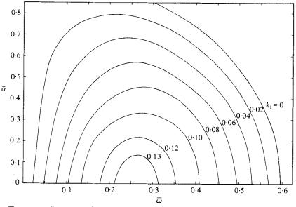
FIGURE 6. Contours of equal  $-k_i$  in the  $\overline{\omega}$ ,  $\overline{\alpha}$  plane showing the unstable region.
