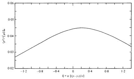
FIGURE 17. Distribution of root-mean-square pressure fluctuations across the mixing layer. (No data available in the literature for comparison.)
