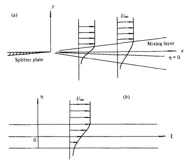
FIGURE 5. Mapping of the mixing layer into the  $\xi$ ,  $\eta$  plane where the turbulence is stationary random. (a) Physical co-ordinates. (b) Similarity co-ordinates.
