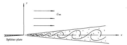
FIGURE 2. Idealized two-dimensional incompressible fully developed turbulent mixing layer with no intrinsic length and time scales.
