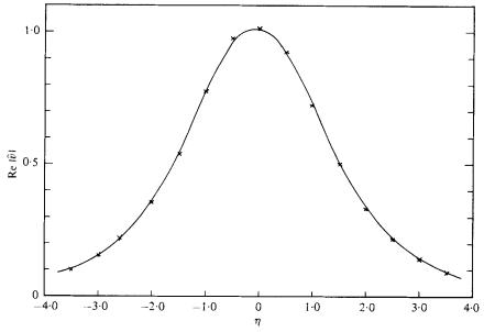
FIGURE 7. Effect of turbulent Reynolds number on the real part of the eigenfunction,  $\overline{\alpha} = 0.5, \ \overline{\omega} = 0.425, \ \dots, R_T = 500; \ \times \dots \times, R_T = \infty.$
