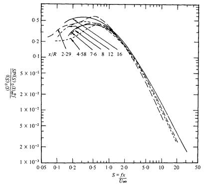
FIGURE 3. Normalized longitudinal turbulent spectra at various axial distances downstream of the nozzle exit of a 3.5 in. diameter jet at approximately one radius from the centre-line. Flow Mach number is 0.3. Data taken from Laurence (1956).
