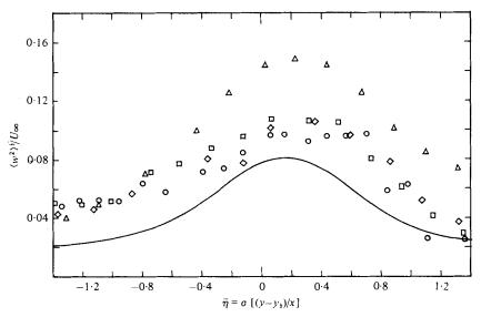
FIGURE 16. Comparison of measured and calculated distribution of root mean square lateral turbulent velocity fluctuations. Patel (1973):  $\diamondsuit$ , x = 28 cm;  $\Box$ , x = 65.3 cm;  $\bigcirc$ , x = 102.5 cm.  $\triangle$ , Wygnanski & Fiedler (1970); -----, present calculation.
