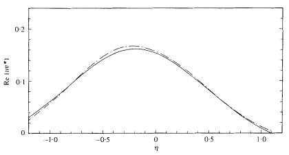
FIGURE 9. A comparison of the distributions of Reynolds stress computed using: —, the full Orr-Sommerfeld equation; --, the Rayleigh equation for  $\hat{v}$  and p and equation (2.9b) for  $\dot{a}$ ;  $R_T = 500, \bar{\alpha} = 0, \bar{\omega} = 0.105$ .
